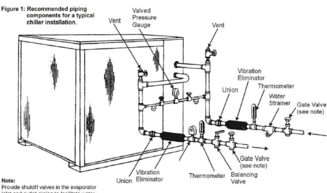
inlet and outlet piping to facilitate water temperature sensor removal.
