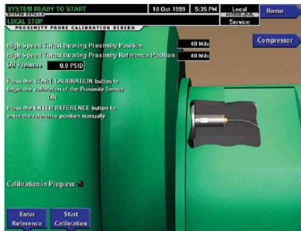
Gear-shaft proximity probe provides a monitoring capability for ultimate assurance of drive line reliability.
