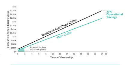
\*Assumptions: 800 ton (2810 kW) chiller operating 24/7 with medium building load, at \$.10kW/hour with no demand charge.
