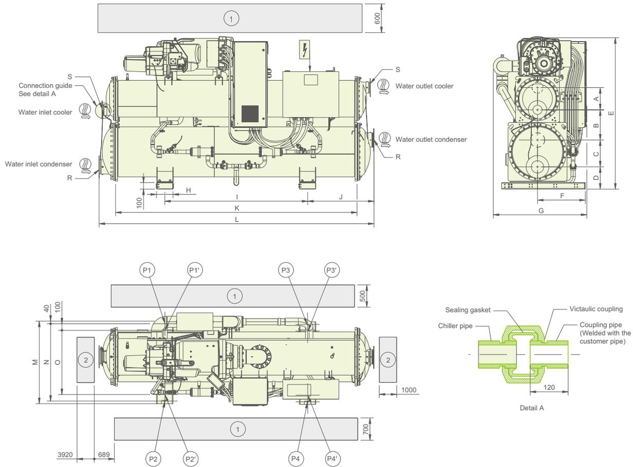
Note: Above chiller condenser and evaporator are 3 passes design
